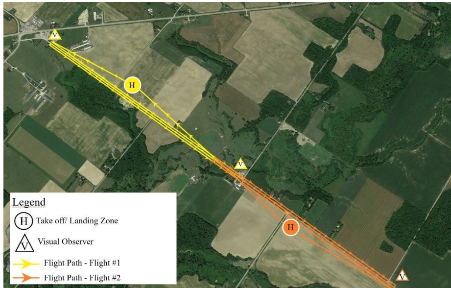
Fig. 4. Path planning for Amiens Rd UAV-based inspection.
